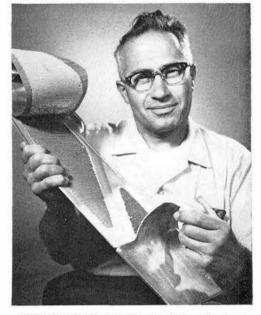
NICK DELOLLIS (1133), Sandia's adhesives authority, displays a sample of structural fabrication using aluminum honeycomb bonded with adhesives to thin aluminum walls. Results of a destructive "peel strength" test show that the aluminum failed before the adhesive. Note the honeycomb metal still adhered to upper peeledback portion.
